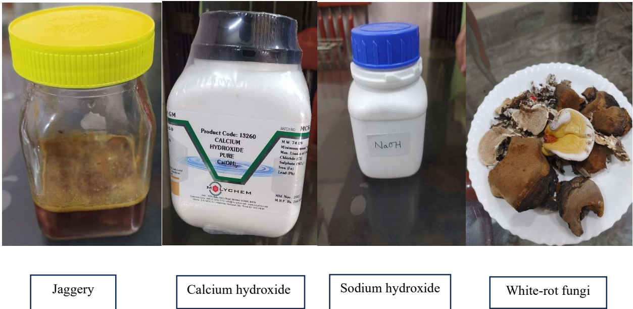
Fig. 4: \text{Ca}(\text{OH})_2 , \text{NaOH} , Jaggery, and White-rot fungi used as additives in reactors- R1 and R2.
