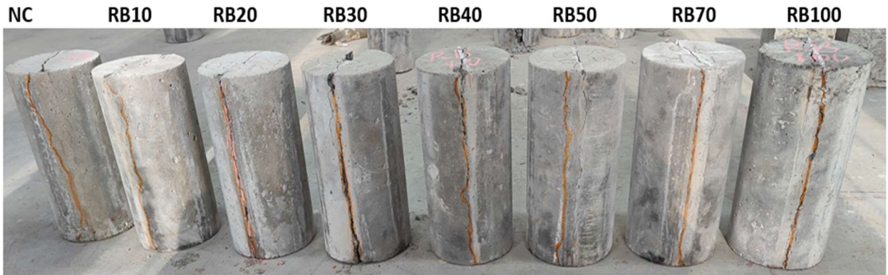
Fig. 13: Failure pattern of cylinder samples at different RB sand content.
