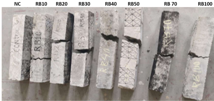
Fig. 15: Failure pattern of prism sample at various RB sand content.
