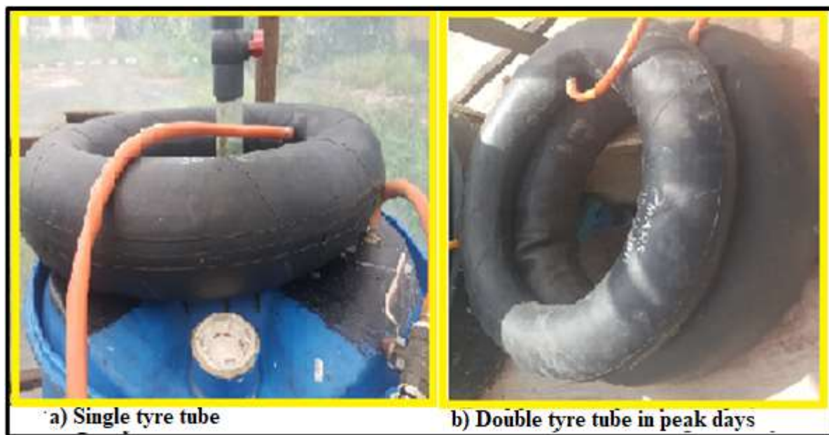
Fig. 3: Biogas-filled 175/65 R14 tyre tube.
