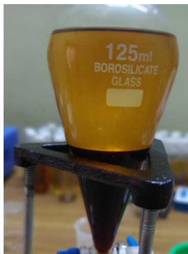
Fig. 3a: Shows two layers of upper layer of biodiesel and the bottom layer of glycerol.
