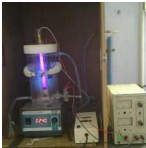
Fig. 1: Schematic diagram of the experimental setup for photoelectrocatalytic reactor.
