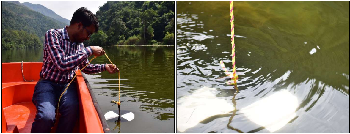
Fig. 2: Use of Secchi disk in the Renuka Lake.
