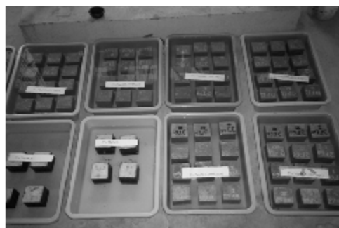
Fig. 10: Curing of specimens in water, magnesium sulphate and sodium sulphate solutions.
