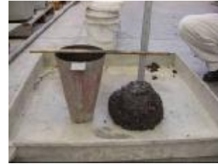
Fig. 3: Workability test-slump cone.
