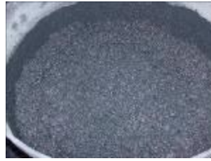
Fig. 2: Fresh geopolymer concrete.
