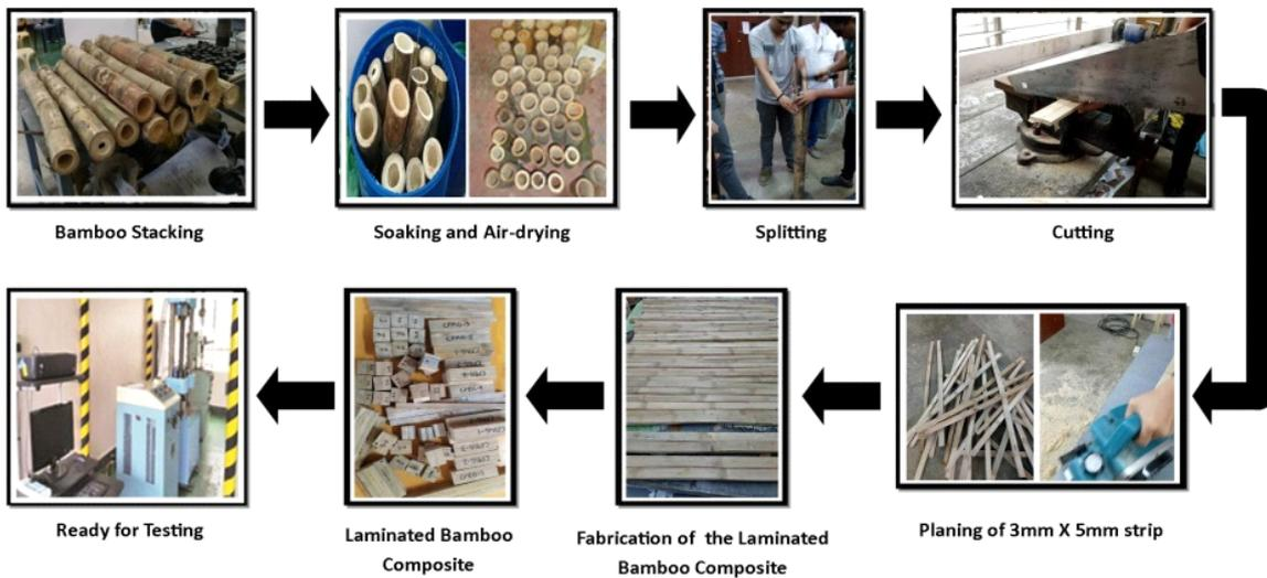
Fig. 2: Distribution flow of laminated bamboo composite.
