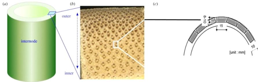
Fig. 1: Extraction of specimens (cross section of bamboo).
