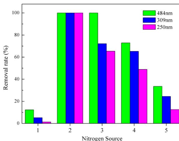
Fig. 3: Effect of various nitrogen sources on degradation of AO7 (20 mg/L). 1: no nitrogen source; 2: yeast extract; 3: peptone; 4: urea; 5: ammonium nitrate.
