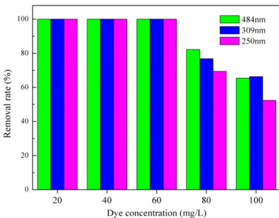
Fig. 6: Effect of initial dye concentration on AO7 degradation.
