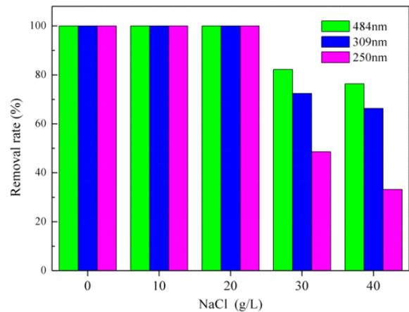
Fig. 7: Effect of NaCl concentration on AO7 degradation.
