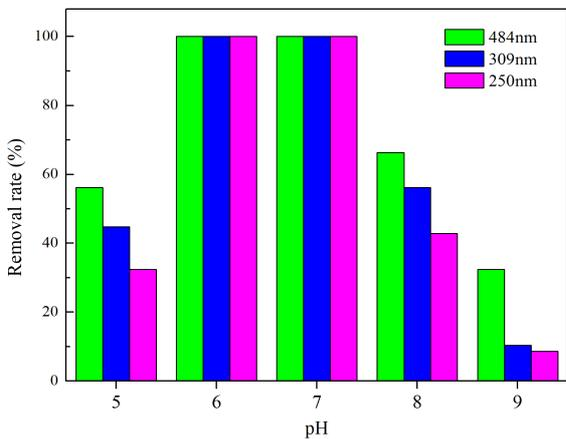
Fig. 5: Effect of pH on AO7 degradation.
