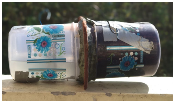
Fig. 2: The MFC reactor constructed from locally sourced material. Here the anode (graphene) is on the right side and has the biodieselwastewater (with aluminum/graphene as the electrode) and the cathode is on the left, the separator is the earthen pot membrane.
