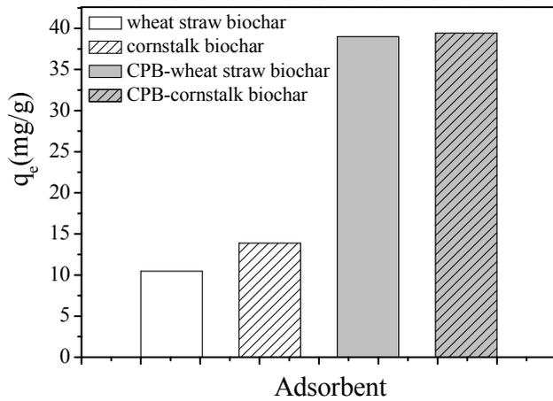
Fig. 1: Adsorption of ORII by the raw and CPB modified biochars.
