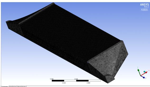
Fig. 2a: Meshed axial flow DOC model.
