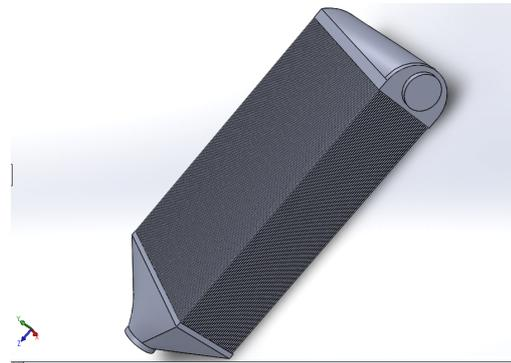
Fig. 1b: Radial flow DOC model.
