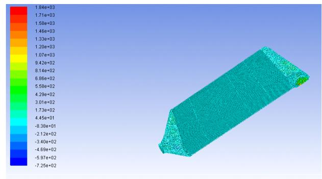
Fig. 10: Contour of radial velocity for radial flow DOC.
