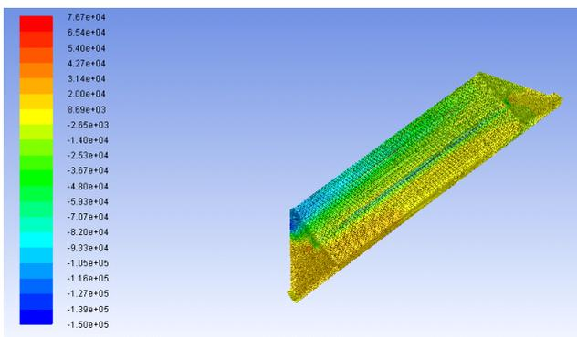
Fig. 3: Contour of pressure coefficient for axial flow DO.
