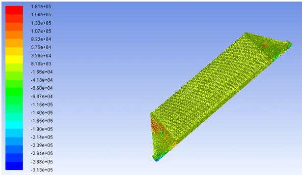
Fig. 5: Contour of axial velocity for axial flow DOC.
