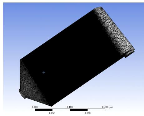
Fig. 2b: Meshed axial flow DOC model.
