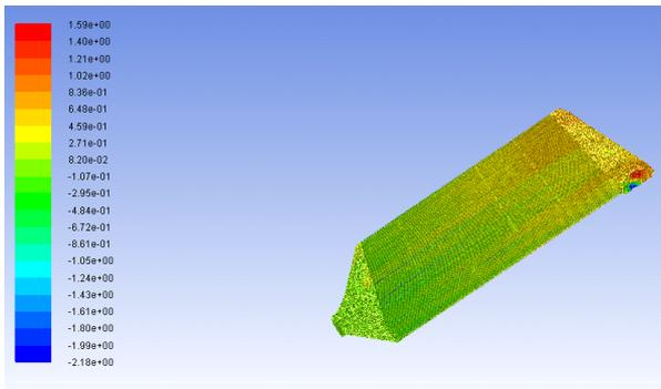
Fig. 9: Contour of pressure coefficient for radial flow DOC.
