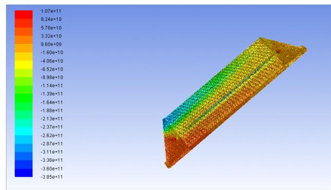
Fig. 4: Contour of total pressure for axial flow DOC.
