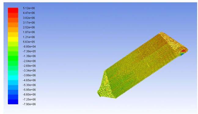
Fig. 8: Contour of total pressure for radial flow DOC.
