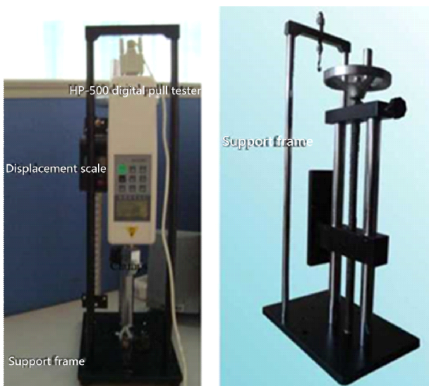
Fig. 2: Pictures of tensile apparatus and its support frame.
