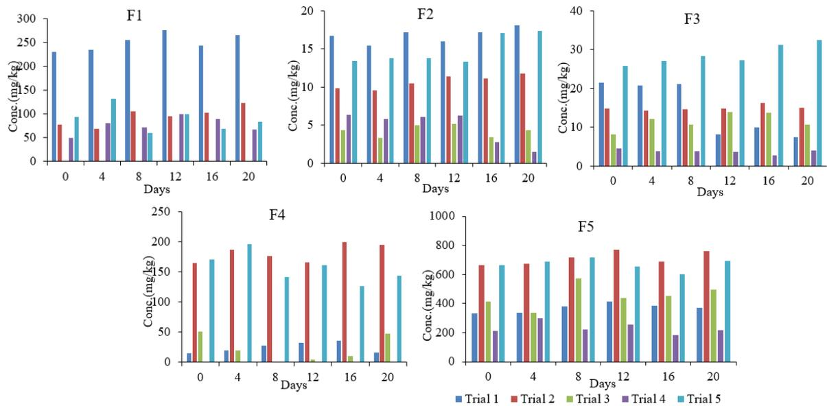
Fig. 2: Speciation of Cd in trial 1, 2, 3, 4 and 5 during the composting process.
