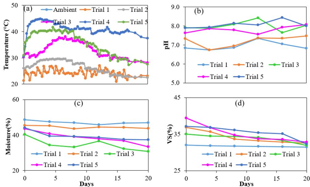
Fig. 1: Variation in physico-chemical parameters during rotary drum composting: temperature (a), pH (b), moisture content (c) and volatile solid, VS (d).
