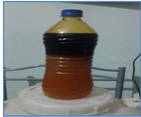
Fig. 6: Phase separation: bio-oil and viscous liquid.
