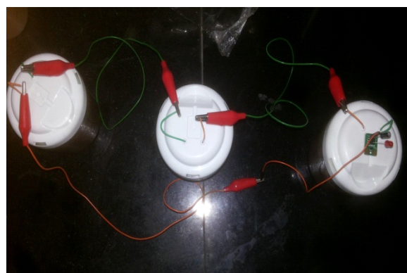
Fig. 2: Three MFCs connected in series.
