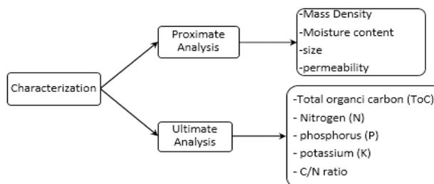
Fig. 3: Characterization of pre-processed waste.
