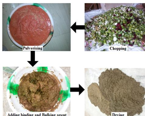
Fig. 2: Stages involved in pre-processing of waste.
