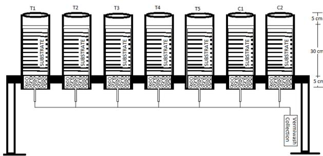
Fig. 4: Schematic representation of the vermi bins.
