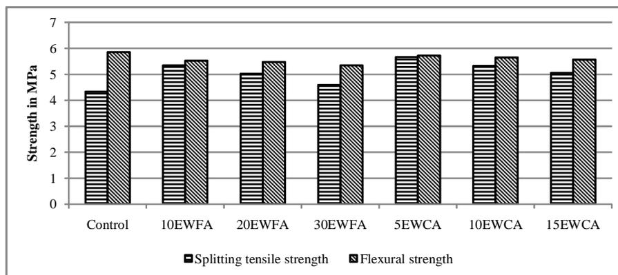
Fig. 7: Splitting tensile strength and flexural strength at 28 days.
