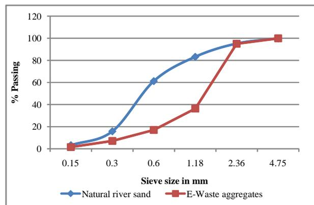
Fig. 2: Sieve analysis of river sand and e-waste fine aggregates.
