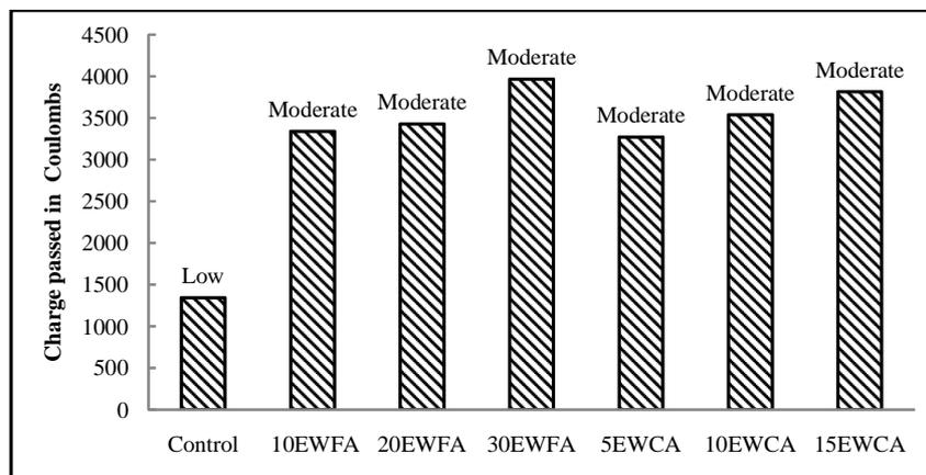
Fig. 8: Rapid chloride ion penetration of control and E-waste concrete mixtures.
