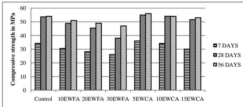
Fig. 4: Compressive strength of control and fiber reinforced green concrete.
