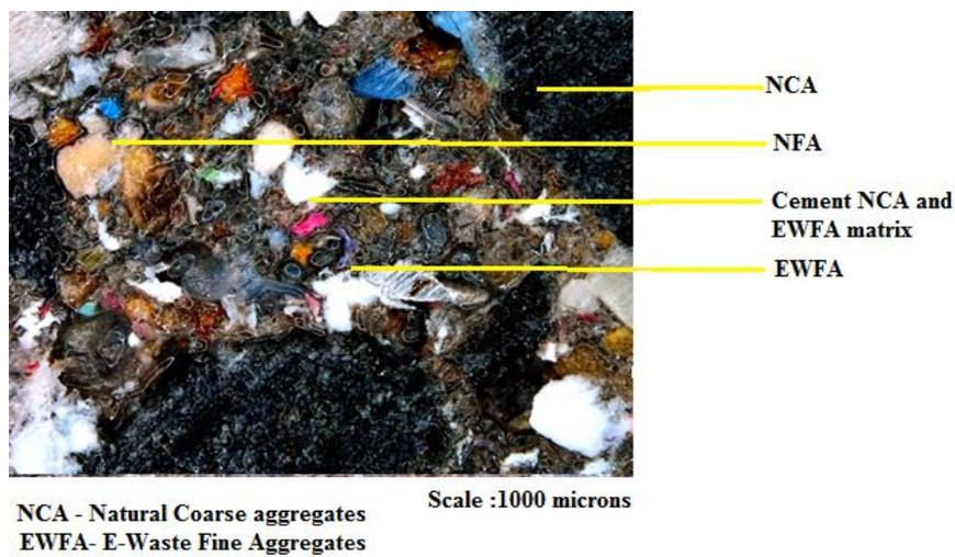
Fig. 5: Electron microscope image of E-waste fine aggregate mixture.
