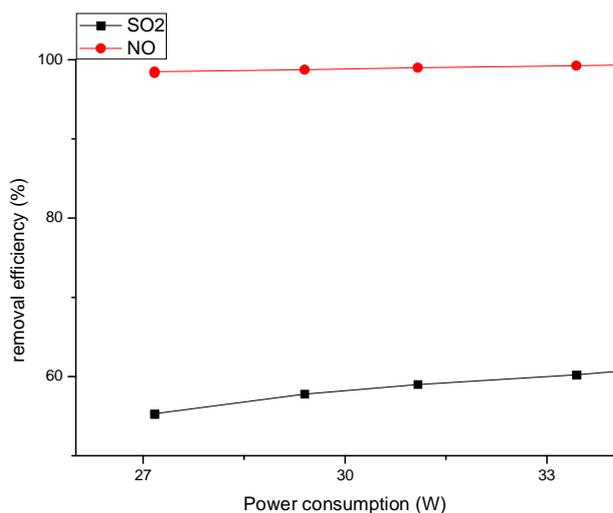
Fig. 5: Analysis of  $\text{NO}_x^-$  and  $\text{SO}_2^-$  removal from flue gas by indirect oxidation.
