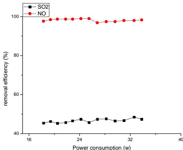
Fig. 6: Analysis of the removal efficiencies of simultaneous indirect desulfurization and denitration.
