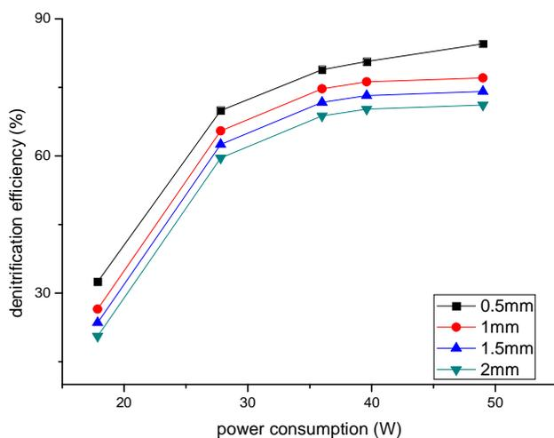
Fig. 7: Analysis of NOx removal from flue gas by the different thickness of the plasma generator.
