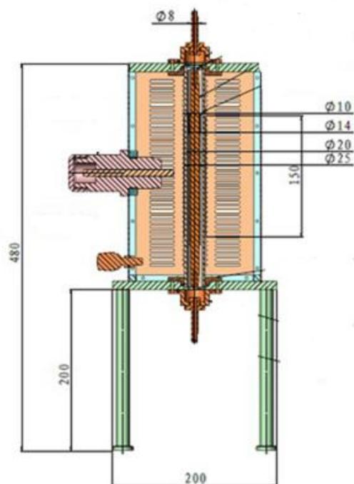
Fig. 1: Structure of the plasma generator.
