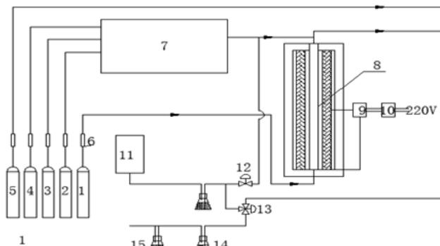
Fig. 3: System used for indirect NTP desulfurization and denitration. The numerals used in the figure are: 1: O<sub>2</sub> bomb, 2: SO<sub>2</sub> bomb, 3: N<sub>2</sub> bomb, 4: NO bomb, 5: NH<sub>3</sub> bomb, 6: flow counter, 7: gas mixer, 8: plasma generator, 9: plasma electric source, 10: voltage transformer, 11: gas analysis equipment, 12: valve, 13: three-way valve, 14: inverted bottle, and 15: dry bottle.
