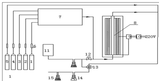
Fig. 2: System used for direct NTP desulfurization and denitration. The numerals used in the figure are: 1:  $O_2$  bomb, 2:  $SO_2$  bomb, 3:  $N_2$  bomb, 4:  $NO$  bomb, 5:  $NH_3$  bomb, 6: flow counter, 7: gas mixer, 8: plasma generator, 9: plasma electric source, 10: voltage transformer, 11: gas analysis equipment, 12: valve, 13: three-way valve, 14: inverted bottle, and 15: dry bottle.
