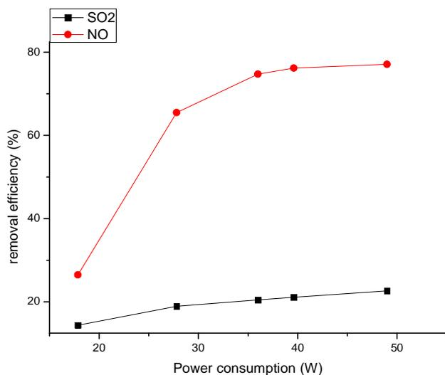
Fig. 4: Analysis of  $\text{NO}_x^-$  and  $\text{SO}_2^-$  removal from flue gas by direct oxidation.
