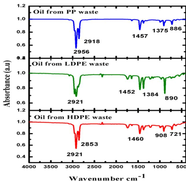
Fig. 2: FTIR spectrum of liquid fuel obtained with HDPE, LDPE, PP.
