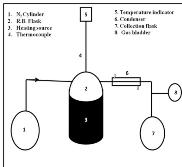
Fig. 1: Pyrolysis experimental setup.
