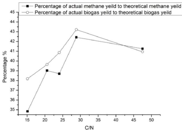
Fig. 7: Performance of anaerobic digestion at different ratios of carbon to nitrogen.
