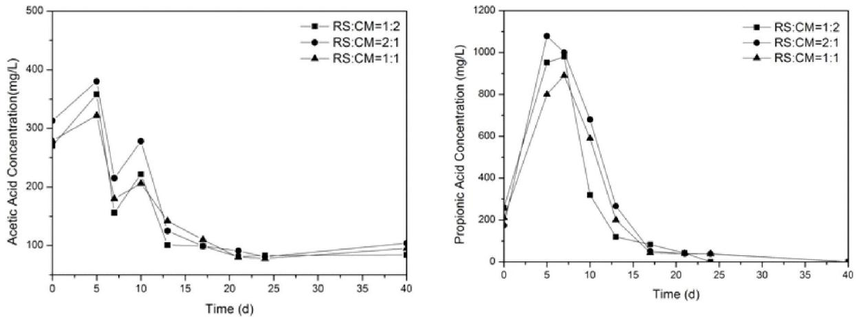
Fig. 5: Dominant VFA concentrations in co-digestion reactors.
