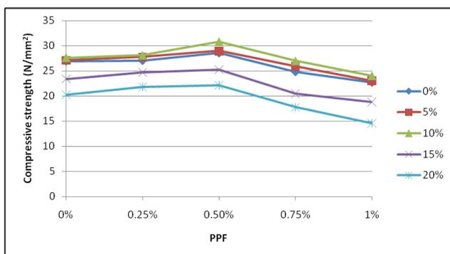
Fig. 4: Compressive strength of different mixes at 28 days.
