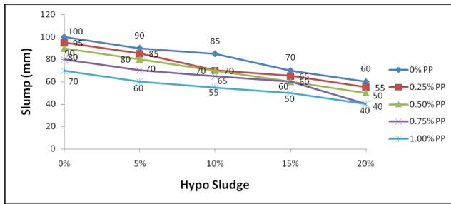
Fig. 1: Degree of workability of various mixes using slump test.
