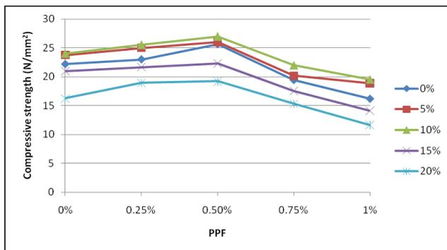
Fig. 3: Compressive strength of different mixes at 14 days.
