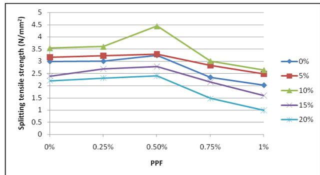
Fig. 6: Splitting tensile strength of different mixes at 14 days.
