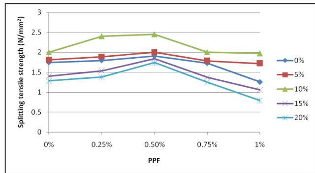
Fig. 5: Splitting tensile strength of different mixes at 7 days.
