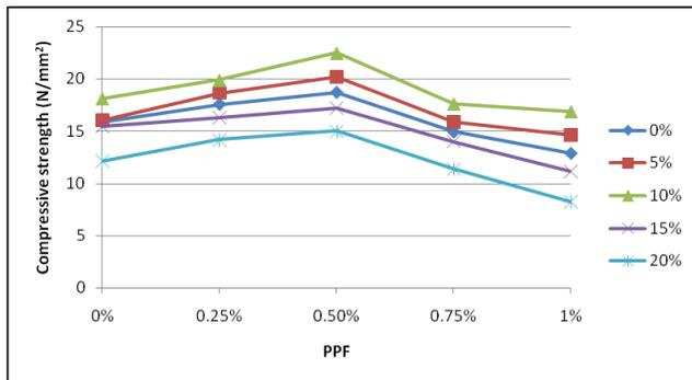
Fig. 2: Compressive strength of different mixes at 7 days.
