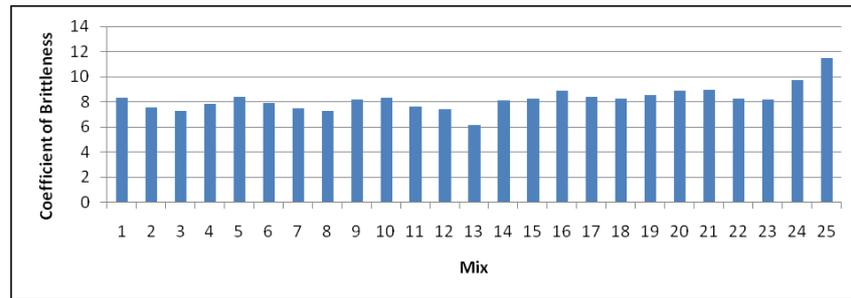
Fig. 8: Variation of coefficient of brittleness for different mixes at 28 days of curing.
