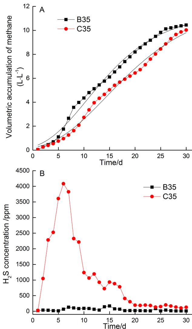
Fig. 3: Methane production and hydrogen sulphide concentration in the 35°C reactor with biochar (B35) and the 35°C reactor without biochar (C35).
