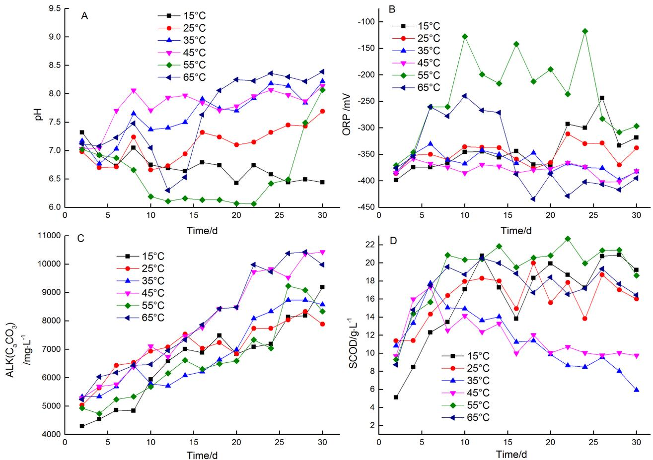
Fig. 2: Process parameters for the anaerobic digestion of chicken manure with biochar under different temperatures.
