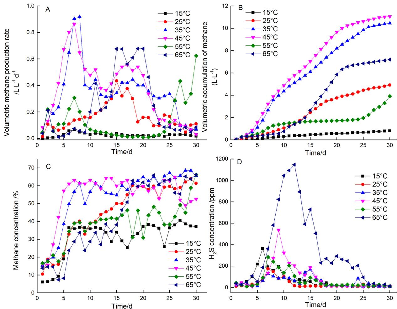
Fig. 1: Methane production, methane and hydrogen sulphide concentration during digestion of chicken manure with biochar at various temperatures.
