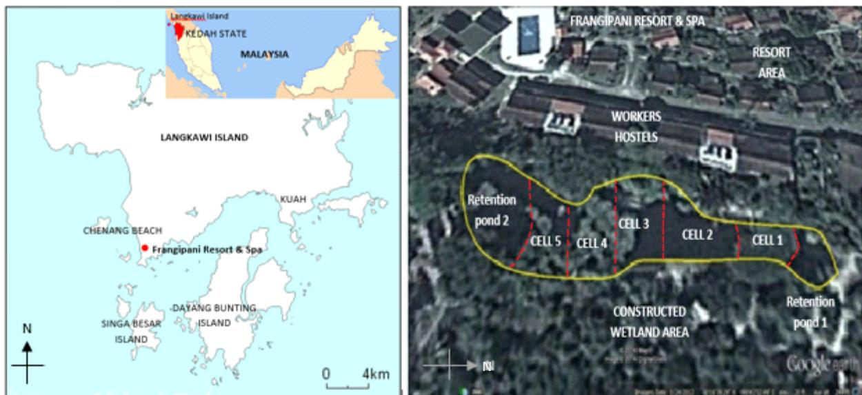
Fig. 1: Left: The location of Frangipani resort & spa at Langkawi Island; Right: The CW system at the backyard of the resort (Source: Google Earth & Google Maps).
