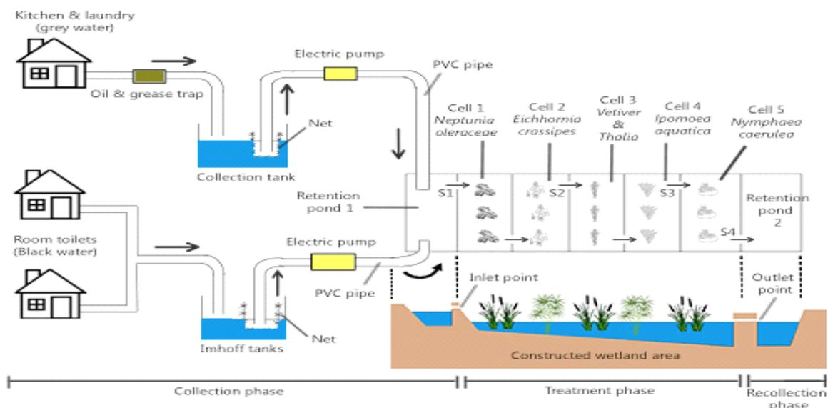
Fig. 2: Layout and wastewater flow of Frangipani Resort constructed wetland system.
