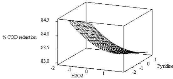
Fig. 2a: Surface plot of [H<sub>2</sub>O<sub>2</sub>] and [pyridine] towards % COD reduction.
