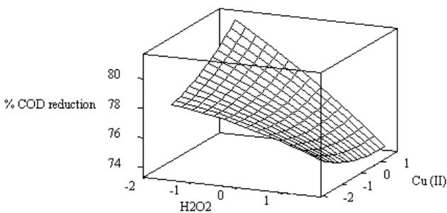
Fig. 4b: Surface plot of [H<sub>2</sub>O<sub>2</sub>], and [Cu (II)] towards % COD reduction.
