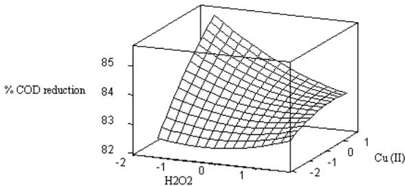
Fig. 2b: Surface plot of [H<sub>2</sub>O<sub>2</sub>] and [Cu (II)] towards % COD reduction.
