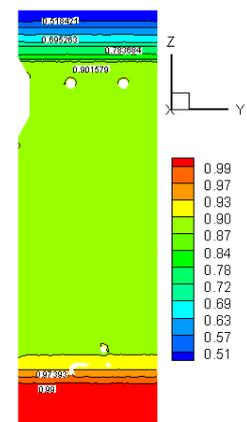
Fig. 14: Aqueous phase concentration distribution of the improved tank.
