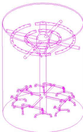
Fig. 12: Physical model of the improved tank.
