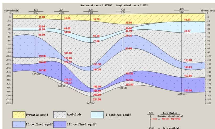
Fig. 2: Confined groundwater burial conditions schematic.
