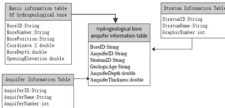
Fig. 4: Hydro-geological bore database structure.
