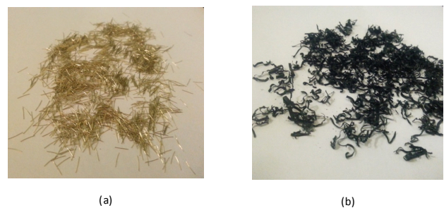
Fig. 1: (a) Micro-steel fiber and (b) recycled HDPE fibers used in SCC mixtures.
