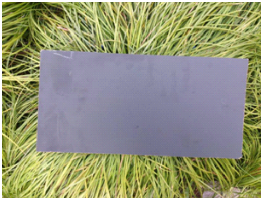
Fig 4: The sample collector for “gypsum rain” measurement.
