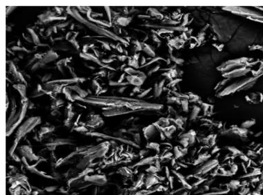
Fig. 2: SEM micrograph of the camphor sawdust.
