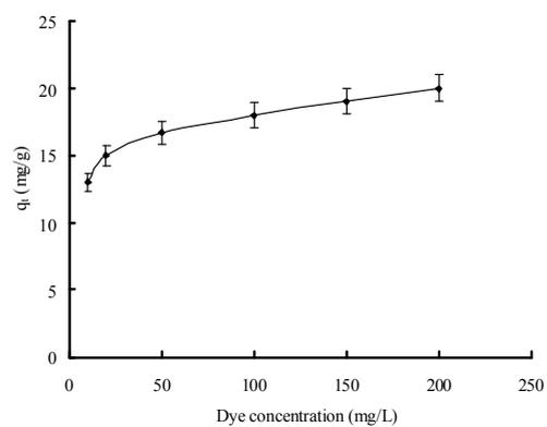
Fig. 6: The influence of dye Congo red concentration on adsorption.
