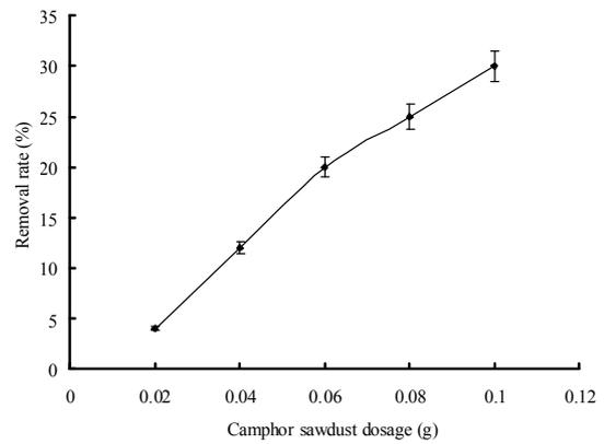
Fig. 5: The influence of camphor sawdust dosage on adsorption.
