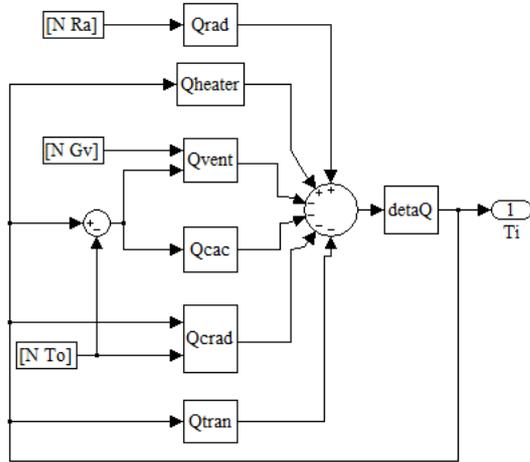
Fig.1: The simulink simulation model of temperature in greenhouse.
