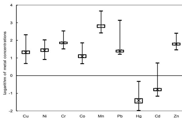
Fig. 2: Variations of potentially toxic elements concentrations after logarithmic transformation (Asterisk stands for median value).
