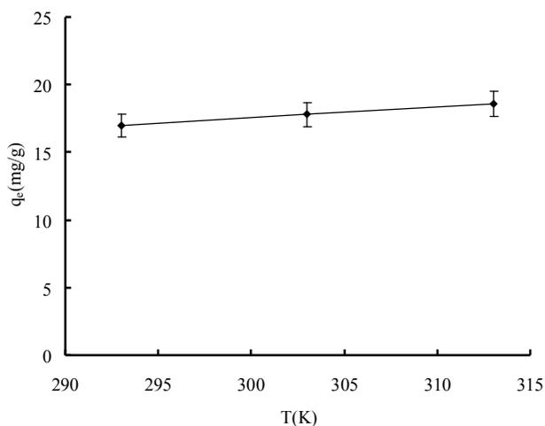
Fig. 5: Effect of temperature on adsorption of dye methylene blue onto activated carbon. Experimental conditions: 0.10 g of activated carbon, 20mg/L of initial dye methylene blue concentration, 120 meshes of particle size, contact time of 200 min, 100 rpm and pH 5.0.
