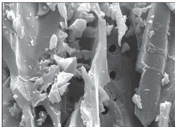
Fig.2: SEM image of activated carbon.
