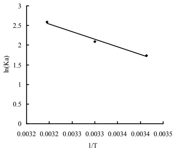
Fig.6: Determination thermodynamic parameters for adsorption of dye methylene blue onto activated carbon. Experimental conditions: 0.10 g of activated carbon, 20mg/L of initial dye methylene blue concentration, 120 meshes of particle size, contact time of 200 min, 100 rpm and pH 5.0.
