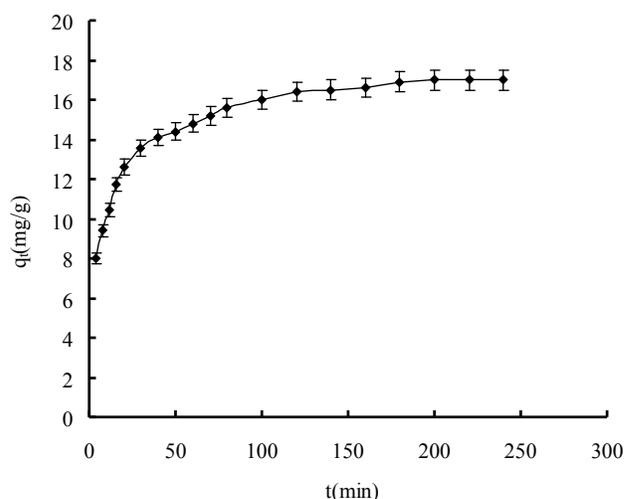
Fig.3: Effect of contact time on adsorption of dye methylene blue in solution onto activated carbon. Experimental conditions: 0.10 g of activated carbon, 20mg/L of initial dye methylene blue concentration, 120 meshes of particle size, 293 K, 100 rpm and pH 5.0.
