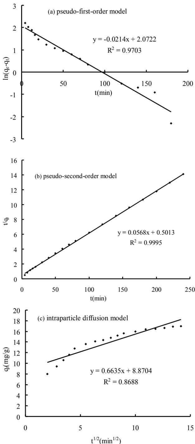
Fig. 4: (a) pseudo-first-order model for adsorption of dye methylene blue onto activated carbon at 293 K. (b) pseudo-second-order model for adsorption of dye methylene blue onto activated carbon at 293 K. (c) intraparticle diffusion model for adsorption of dye methylene blue onto activated carbon at 293K. Experimental conditions: 0.10 g of activated carbon, 20mg/L of initial dye methylene blue concentration, 120 meshes of particle size, 293 K, 100 rpm and pH 5.0.
