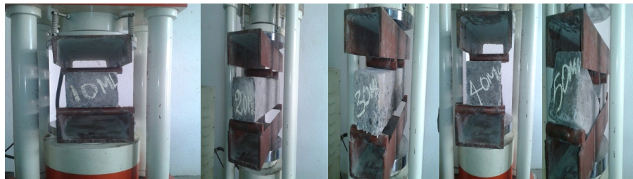
Fig. 7: Flexural strength test with various proportions (10mL, 20mL, 30mL, 40mL, 50 mL) of bacteria.
