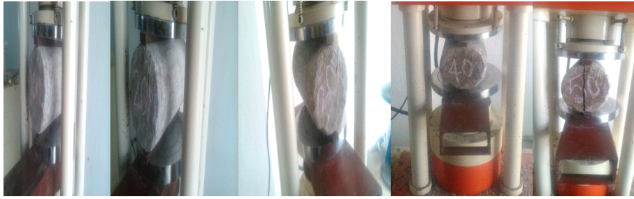
Fig. 6: Split tension test with various proportions (10mL, 20mL, 30mL, 40mL, 50 mL) of bacteria.
