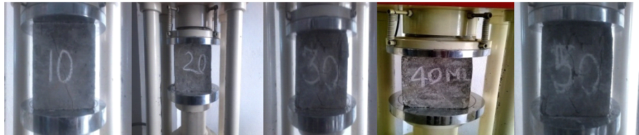
Fig. 3: Testing of compressive strength with various proportions (10mL, 20mL, 30mL, 40mL, 50 mL) of bacteria.
