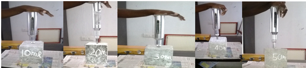
Fig. 4: Testing of rebound hammer with various proportions (10mL, 20mL, 30mL, 40mL, 50 mL) of bacteria.
