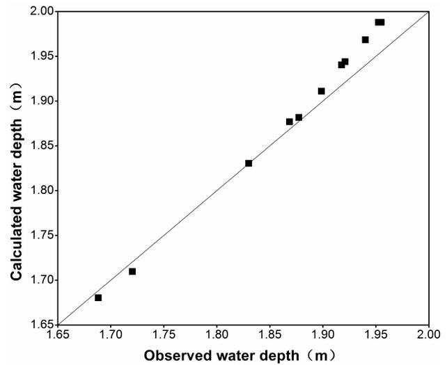
Fig. 4: Measured water depth and calculated depth without silting and scouring.
