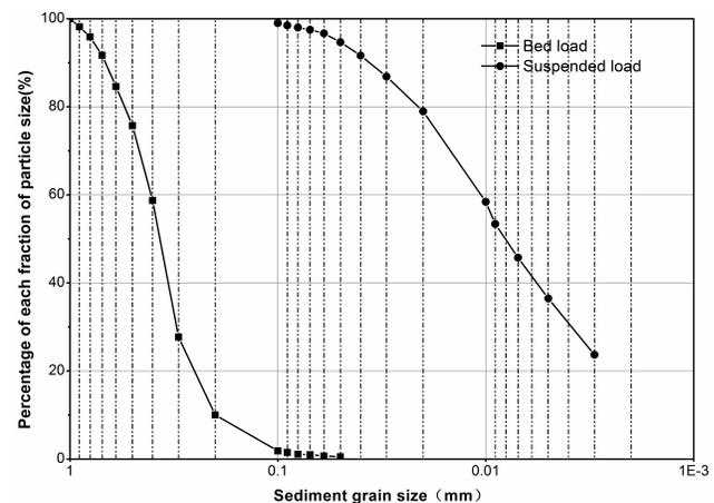
Fig. 2: Sediment gradation of suspended load and bed load.
