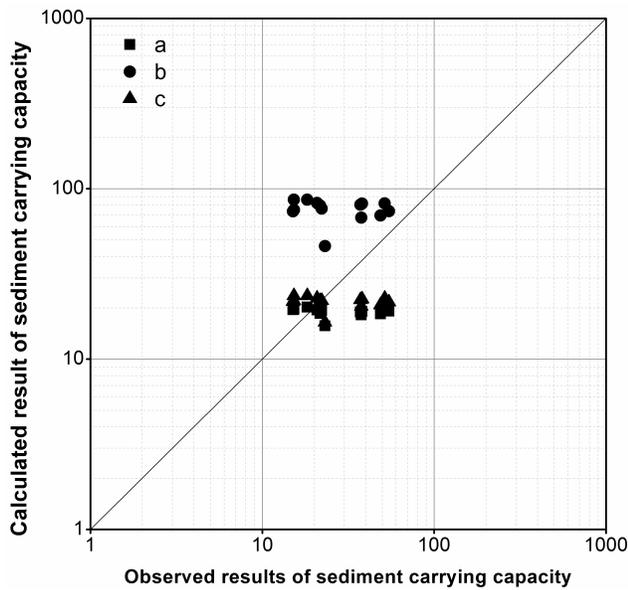
Fig. 3: Comparison of the calculated results of different channel sediment carrying capacity formulas (a - the Yellow River irrigation channel; b - loess irrigation channel; c - Wuhan University Institute of Water Resources and Hydropower) with the measured data.
