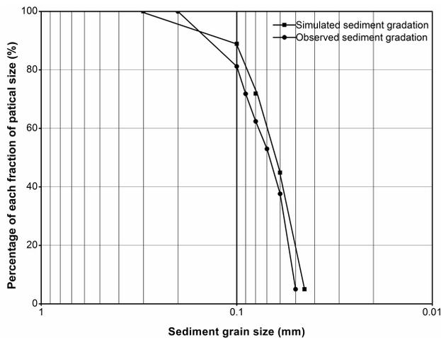
Fig. 5: Comparison of simulated sediment gradation and observed sediment gradation.
