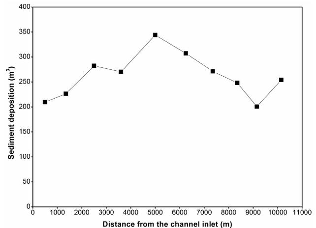
Fig. 6: Sediment deposition and distribution along the channel.
