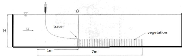
Fig. 2: The sketch of the experimental arrangement.
