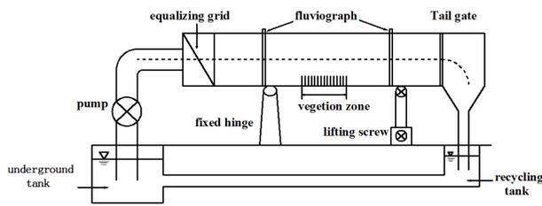
Fig. 1: The experimental re-circulating open-channel rectangle flume setup.
