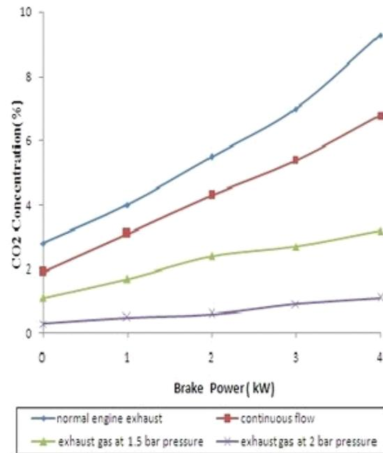
Fig. 3: Variation of CO<sub>2</sub> concentration with respect to brake power.
