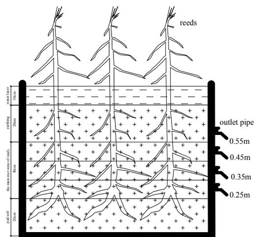
Fig. 1: Cross-section diagram of test device.
