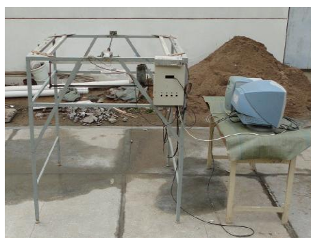
Fig. 2: Homemade laser scanner.
