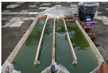
Fig. 2. The paddle wheeled pilot scale bioreactor during the treatment (without cover).
