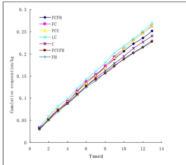
Fig. 1: Cumulative evaporation capacity for each treatment.
