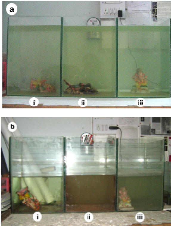
Fig. 1: (a) experimental setup, (b) situation after 5 weeks. (i) Fibre idol, (ii) shadoo idol, (iii) plaster of Paris idol.
