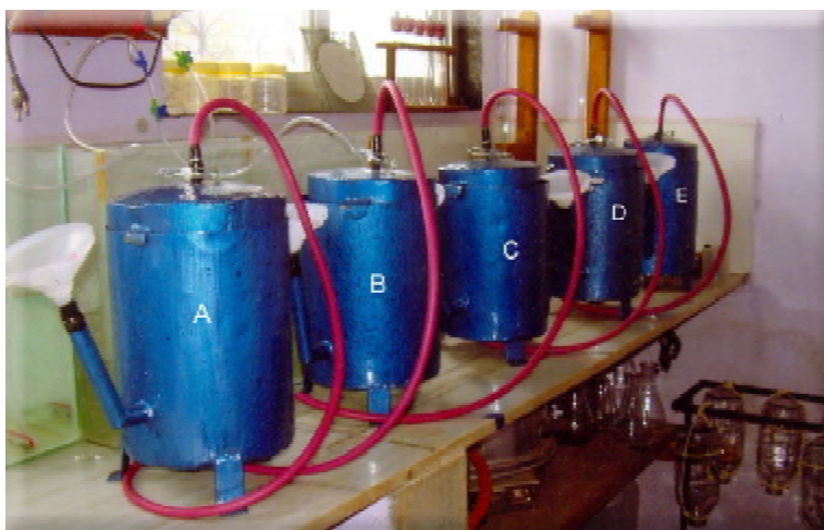
Fig. 1: 1 L capacity biogas digesters in row used for optimization studies.
