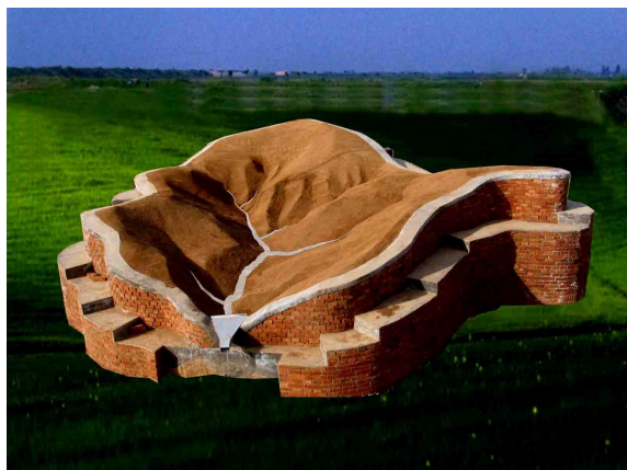
Fig. 3: The 1:100 (the model: the prototype) physical model of the KangJiaGeLao watershed.
