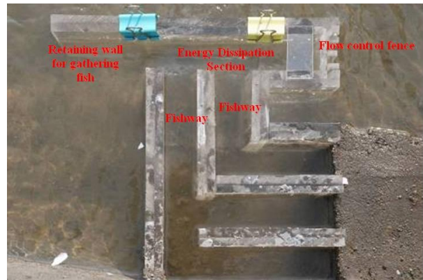
Fig. 2: The device of tempting fish and making up water at fishway inlet.
