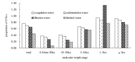
Fig. 10: The organic matter removal of the water of southern Ganjiang River on MV distribution of UV<sub>254</sub>.
