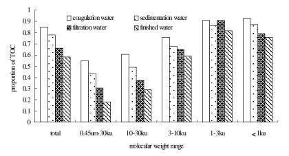
Fig. 9: The organic matter removal of the water of northern Ganjiang River on MV distribution of TOC.
