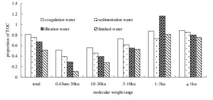
Fig. 11: The organic matter removal of the water of northern Ganjiang River on MV distribution of TOC.
