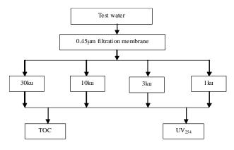
Fig. 1: Determining process of MV distribution of organic matters.
