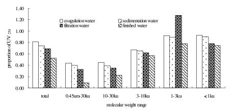
Fig. 8: The organic matter removal of the water of northern Ganjiang River on MV distribution of UV<sub>254</sub>.
