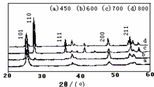
Fig. 9: XRD result of TiO<sub>2</sub> thin film by heat treatment.
