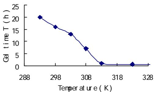
Fig. 7: Effect of hydrolysable temperature on gelable time (with AcAc solvent, n[H<sub>2</sub>O] : n[Ti(OBu)<sub>4</sub>] = 2.5, n[NH(C<sub>2</sub>H<sub>5</sub>OH)<sub>3</sub>] : n[Ti(OBu)<sub>4</sub>] = 1, n[Eth] : n[Ti(OBu)<sub>4</sub>] = 21, pH = 3.5).
