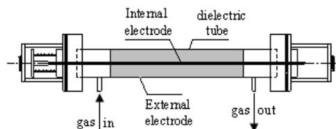
Fig. 2: NTP reactor
