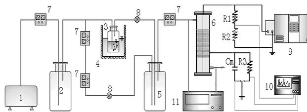
Fig. 1: Schematic diagram of NTP system for benzene removal. 1. air compressor, 2. buffer, 3. benzene liquid bottle, 4. attemperater, 5. blender, 6. NTP reactor, 7. mass flow meter, 8. needle valve, 9. high voltage, 10. oscukkograph, 11. gas chromatograph
