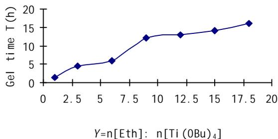
Fig. 5 Effect of solvent quantity on gelable time (With AcAc solvent, n[H<sub>2</sub>O] : n[Ti(OBu)<sub>4</sub>] = 3, n[AcAc] : n [Ti(OBu)<sub>4</sub>] = 1, hypothetically, n[Eth] : n[Ti(OBu)<sub>4</sub>] = Y (Mole ratio), gel time for T).
