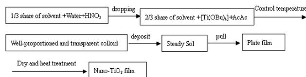
Fig. 3: Flow chart on preparing nano-TiO<sub>2</sub> thin film by sol-gel method.
