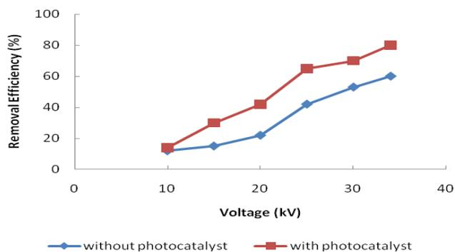
Fig. 10: Comparing benzene removal efficiency with or without photocatalyst in plasma reactor. (benzene concentration is 1500 mg/m<sup>3</sup>, the average voltage is 30 kV and gas flow rate is 14 mm/s)
