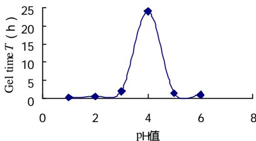
Fig. 6: Effect of pH on gelable time (with AcAc solvent, n[H<sub>2</sub>O] : n[Ti(OBu)<sub>4</sub>] = 2.5, n[NH(C<sub>2</sub>H<sub>5</sub>OH)<sub>3</sub>] : n[Ti(OBu)<sub>4</sub>] = 1, n[Eth] : n[Ti(OBu)<sub>4</sub>] = 21. Through dropping HNO<sub>3</sub> to change pH value, the gelation time T was tested under different pH values).
