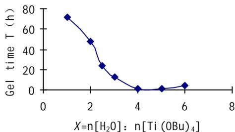
Fig. 4: Effect of water quantity on gelable time (n[Eth] : n[Ti(OBu)<sub>4</sub>] = 21, n[AcAc] : n [Ti(OBu)<sub>4</sub>] = 1, hypothetically, n[H<sub>2</sub>O]:n[Ti(OBu)<sub>4</sub>] = X (Mole ratio), gel time for T).
