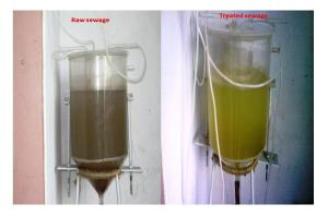
Fig. 2: Raw and treated mixed wastewater.
