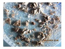
Fig. 3: Struvite crystal formed over the sludge of mixed wastewater with parent seed.
