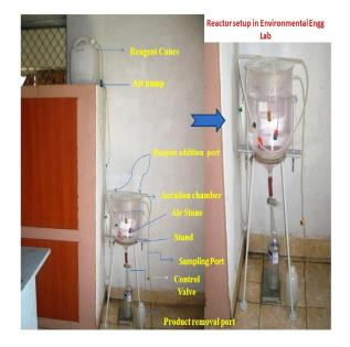
Fig. 1: Reactor setup.
