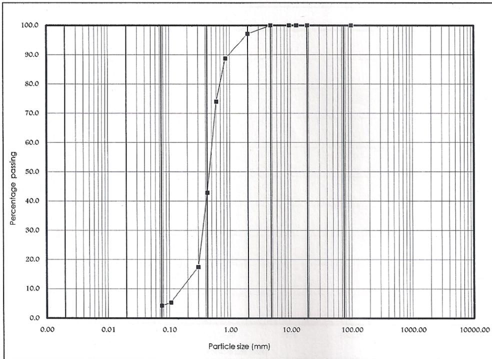
Fig. 7: Particle size distribution curve of BH 1 @ 30.00m.
