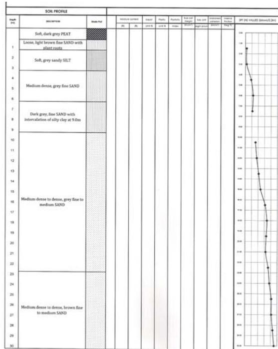
Fig. 3: Log of Borehole 2.
