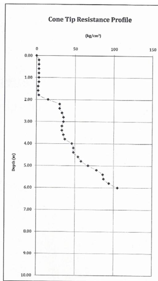
Fig. 6: Penetrometer log of CPT 2.
