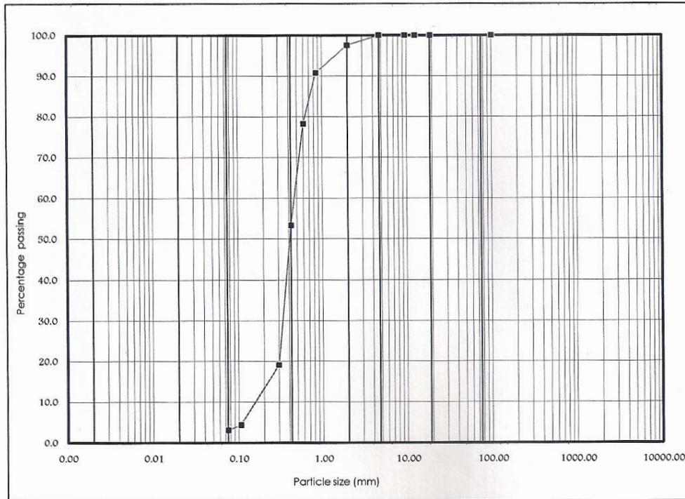
Fig. 9: Particle size distribution curve of BH 3 @ 30.00m.
