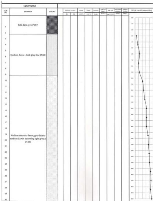
Fig. 2: Log of Borehole 1.
