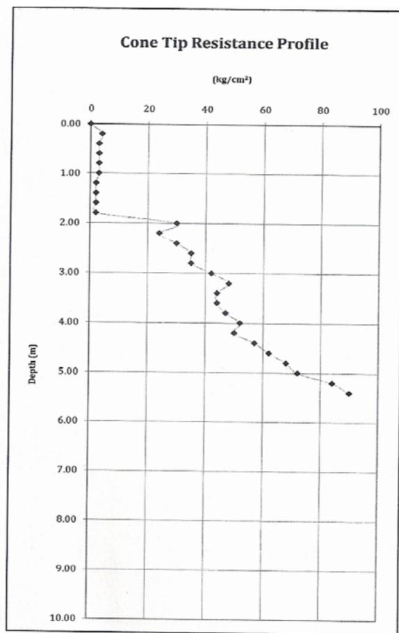
Fig. 5: Penetrometer log of CPT1.
